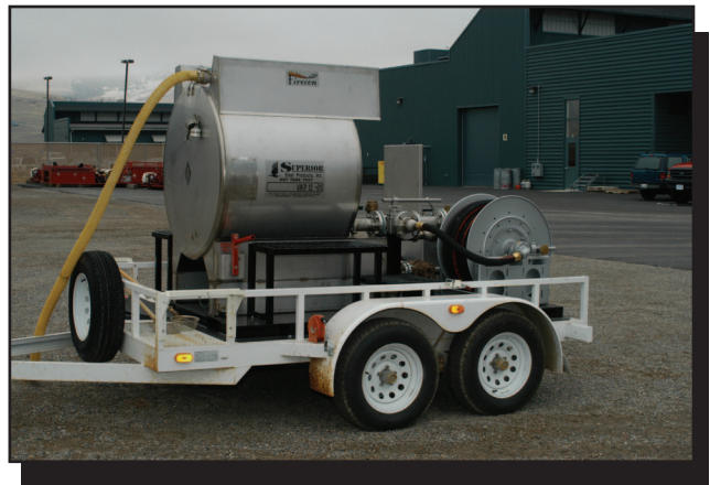
Figure 23—A 240-gallon DOT-406 tank being used as a batch mixer.
