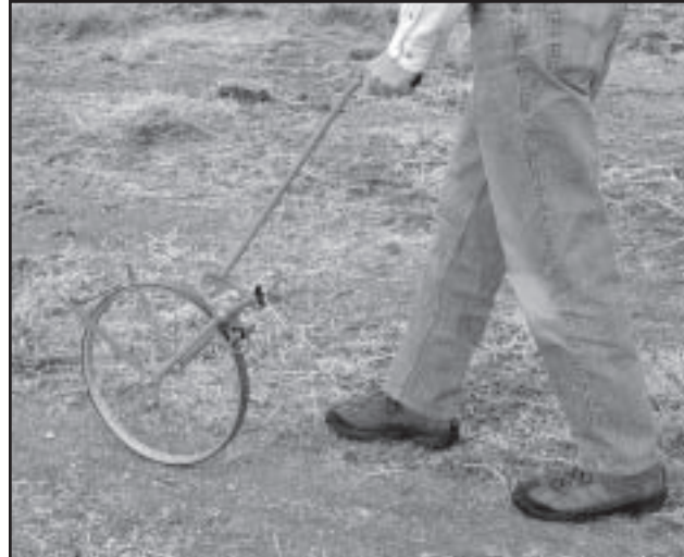
Figure 1—A measuring wheel can be used to measure the distance of the test course.
