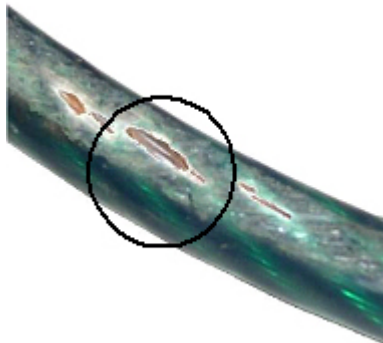
Figure 5. Damaged plastic coated wire rope.
