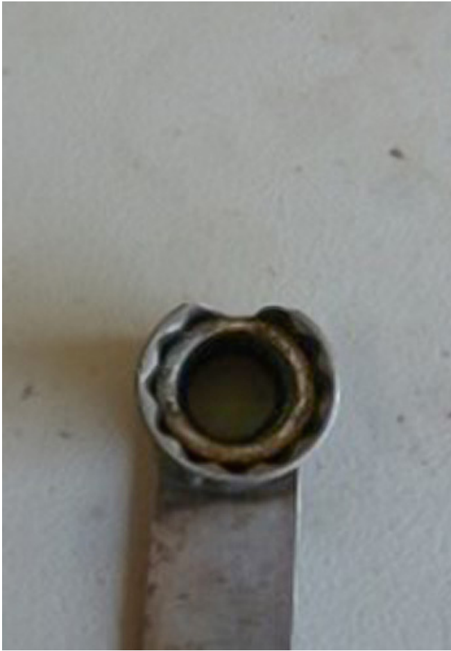
2. Port removal tool close up
