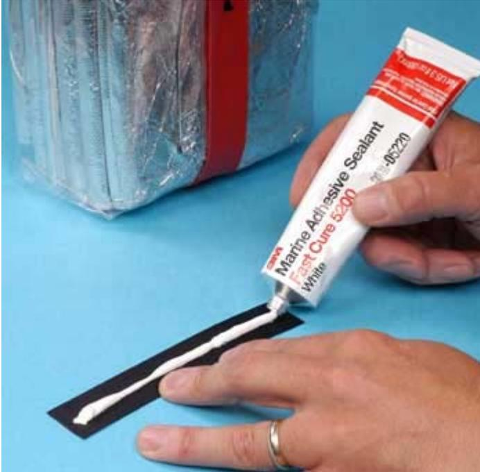
**STEP 1: Perform all work in a well ventilated area. Cut the webbing to proper length with a heat knife or sear the ends with a match to prevent them from fraying. Apply a thin bead of adhesive to the nylon webbing.**
