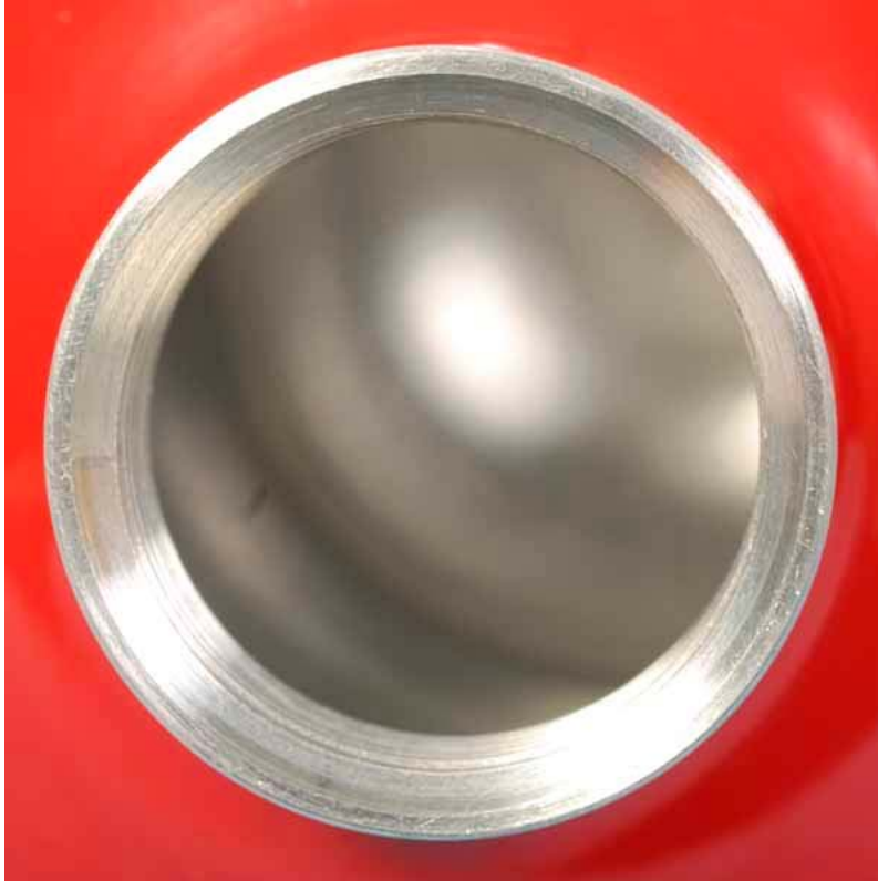
The mouth of a compliant fuel bottle. Note the lack of a crimp line.
