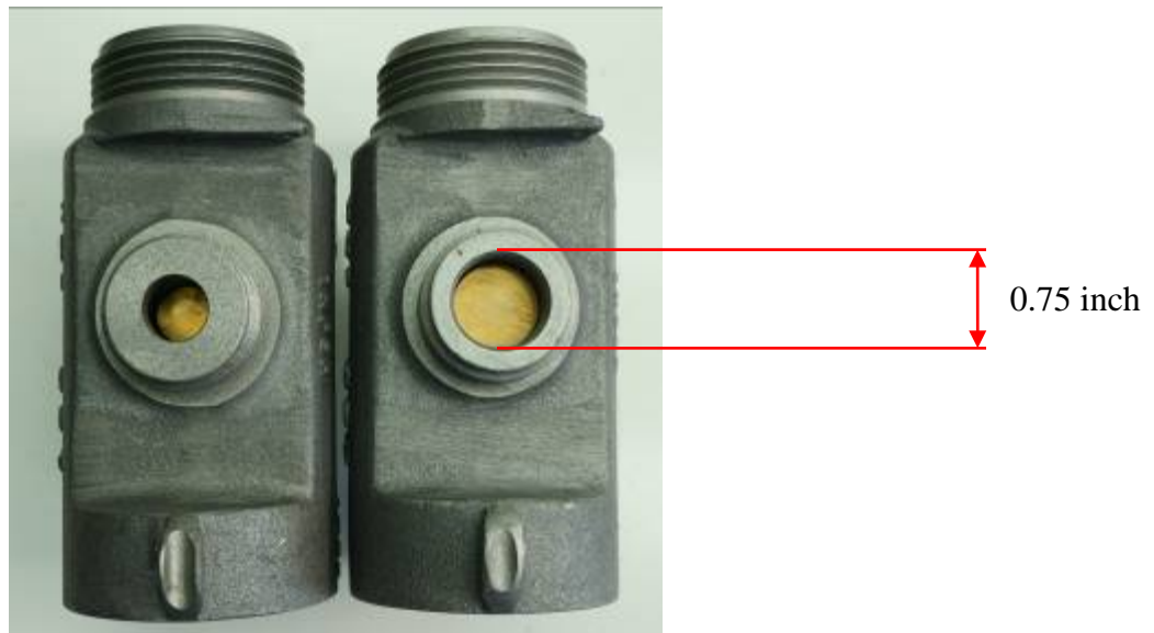
Figure 3--large 0.75 inch diameter on branch waterway for potentially affected tees (right) versus an unaffected tees a (left)
