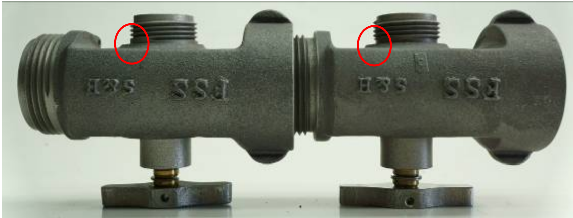
Figure 4--comparison between potentially affected tee (without thread relief; left) and unaffected tee (with thread relief; right)
