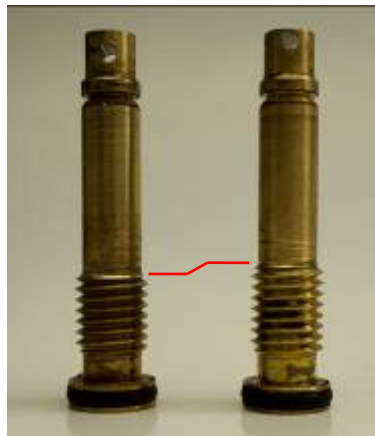
Figure 1— Comparison of threads on the valve stem; nonworking valve (left) and working valve (right). Note that the working valve stem has one full thread more than the nonworking unit
