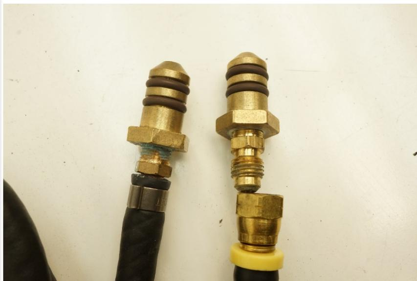
Figure 1—Comparison of fuel lines currently contracted by DLA. The affected fuel line from Waterax is on the right. The unaffected fuel line from Drop Systems is on the left.
