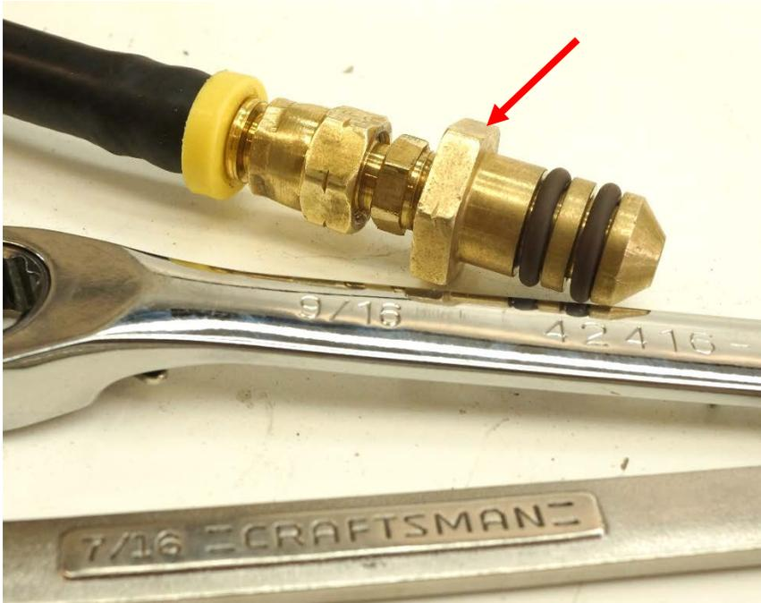
Figure 3—Fuel inlet quick connect after wrench tightening, 1/3 turn past finger tight. Note the full engagement of the threads.
