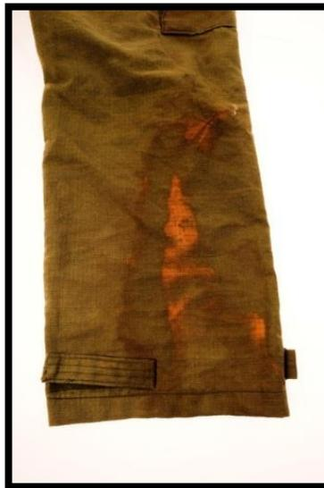
Equipment specialists and engineers from the National Technology and Development Program (T&D) conducted tests using a drip torch, flame resistant (FR) pants, wool-blend socks, and a piece of wood to simulate a leg. T&D performed the experiment to compare the temperatures outside the pants, inside the pants, and inside the sock with burning drip torch fuel on the pants.
