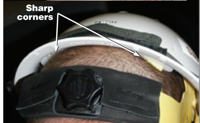
Figure 2—This Bullard hardhat provides adequate space when fully seated on the user's head (top). Less space between the redesigned Bullard hardhat and the user's head can cause pressure points (bottom).
